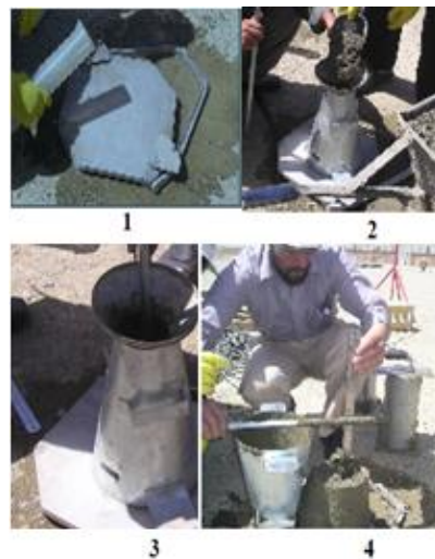
Fig. 4 Performing the slump test after ensuring that the mixture is well mixed.
