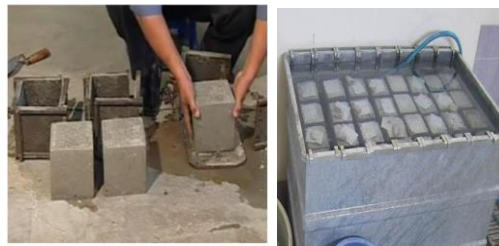
Fig. 7 Removing the molds from the samples and placing them in the water tank
