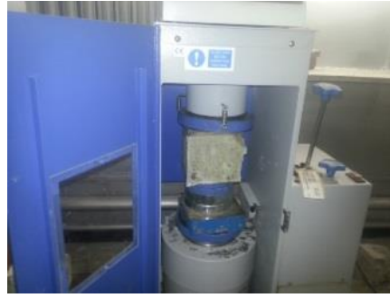
Fig. 8 Determining the Compressive Strength of Cubic Specimens of Concrete
