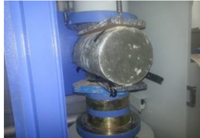
Fig. 9 Splitting Tension Test of a Concrete Cylindrical Specimen
