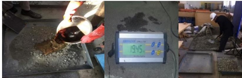
Fig. 3 Weighing and Mixing of Gravel and Sand and Adding Superplasticizer to the Concrete Mixture
