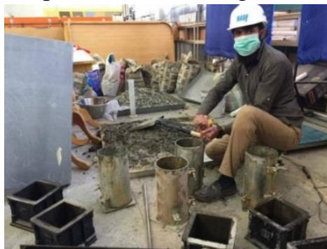
Fig. 5 Checking and lubricating molds for cubic and cylindrical specimens
