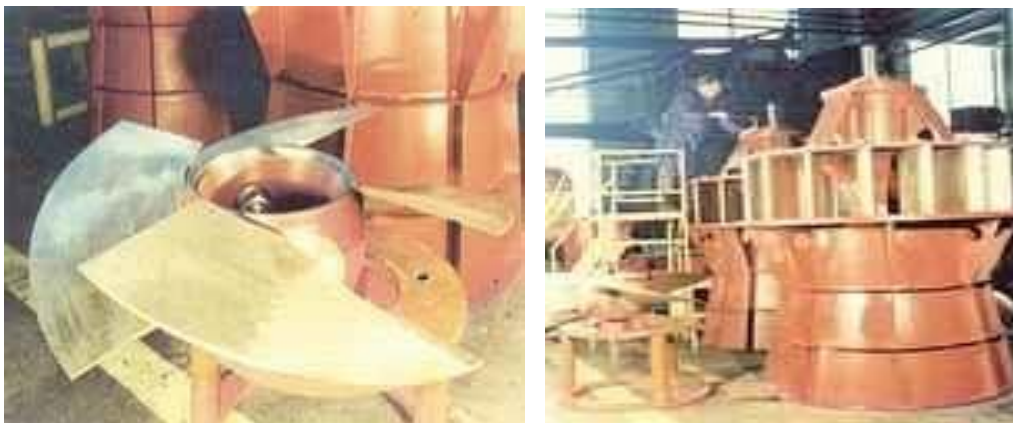
Fig. 5 Axial turbine hydraulic units
